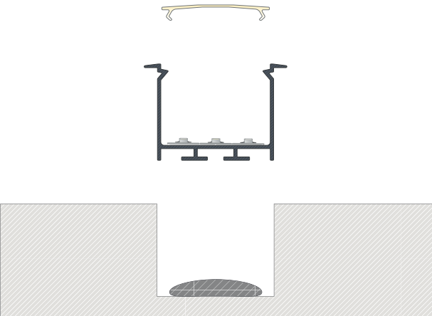
Assembly instructions for the HEDE set in a milled hole using mounting adhesive.
