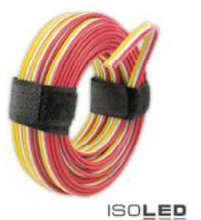
114713 | Cable CCT 25m roll 3-pole 0.75mm 2 H03VH-H AWG18
