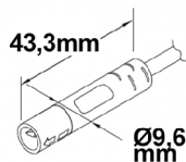
113527 | Mini-Plug connector socket female, 1m, 2x0.75, IP54, white-green,
