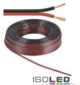
114704 | Cable 25m roll 2-pin 0.75mm² H03VH-H YZWL, black/red, AWG18
