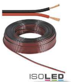
114163 | Cable 50m roll 2-pole 1.5mm 2 H03VH-H YZWL, black/red, AWG16
